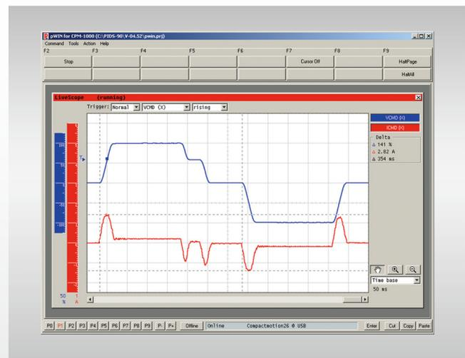
Drive calibration is facilitated by the real-time debugger's Live Scope, which allows observation and analysis of the drive's response characteristics at the computer. One of Live Scope's special features is to display in real-time mode like an oscilloscope, which allows immediate observation of events in the drive system.
